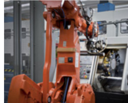
Nine automated turning islands
