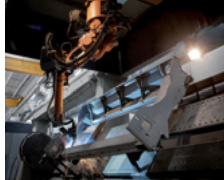
Four automated welding islands
